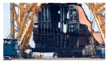
April 28 - On Tuesday, salvors hoisted and removed the engine room section of the grounded ro/ro Golden Ray, loading it onto a deck barge for transport to a recycling facility in Louisiana.
